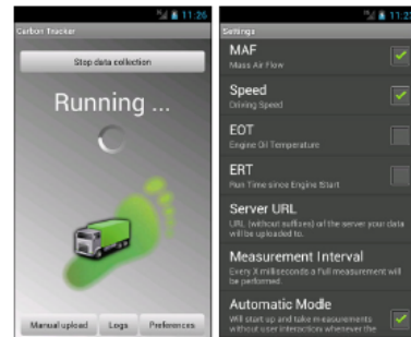
Fig. 4 DCS Android application: running mode and settings
