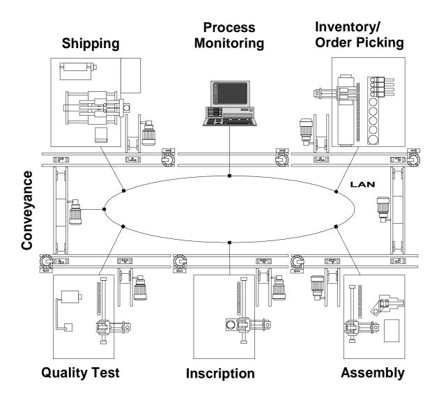
Fig. E.III.03: Concept of the Y-CIM prototype installed in the Y-CIM-Lab at CETEMM Euvaldo Lodi, Rio de Janeiro
