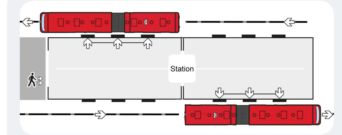
Left: A typical bus station layout, as it exists in many (not only) Latin-American countries. The Trans Milenio System, nevertheless, partly consists of more complex bus stations (right). The stations include two sub-stations, can be accessed by two-plus-two busses and two lanes per direction. On each bus berth various bus lines can halt.
