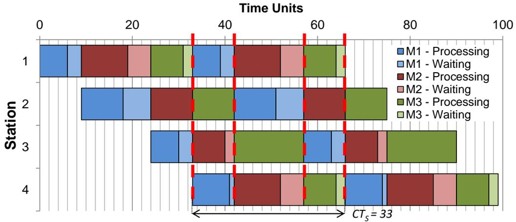
Figure 2: Optimal Cyclical Schedule for a Synchronous Line ( $S_{\text{sync}} = \{1, 2, 3, 4\}$ ), with  $CT_S=33$ .
