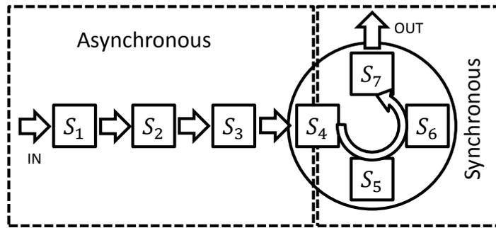
Figure 1: Hybrid unpaced line layout ( $S_{\text{async}} = \{1, 2, 3, 4\}$ ,  $S_{\text{sync}} = \{5, 6, 7\}$ )
