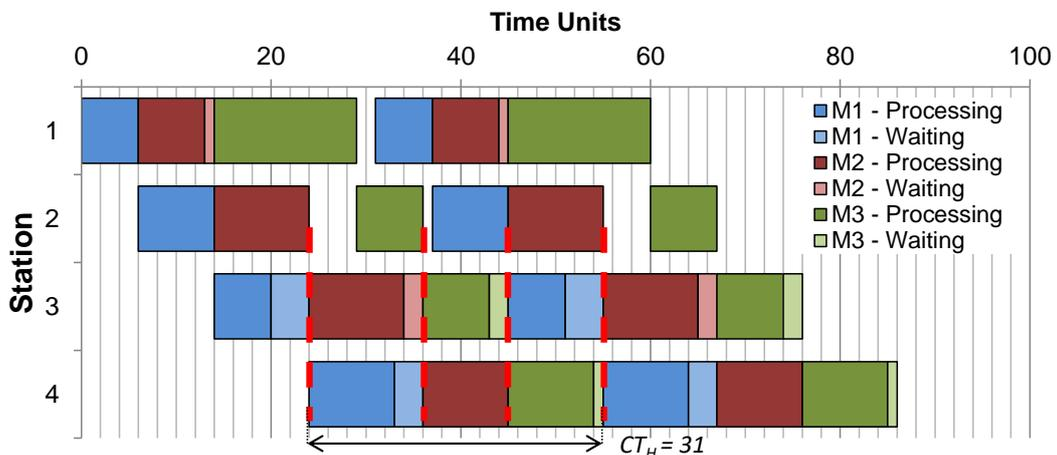
Figure 4: Optimal Cyclical Schedule for a Hybrid Line ( $S_{\text{async}} = \{1, 2\}$ ,  $S_{\text{sync}} = \{3, 4\}$ ), with  $CT_H=31$ .
