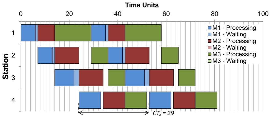
Figure 3: Optimal Cyclical Schedule for an Asynchronous ( $S_{\text{async}} = \{1, 2, 3, 4\}$ ) Line, with  $CT_A=29$ .
